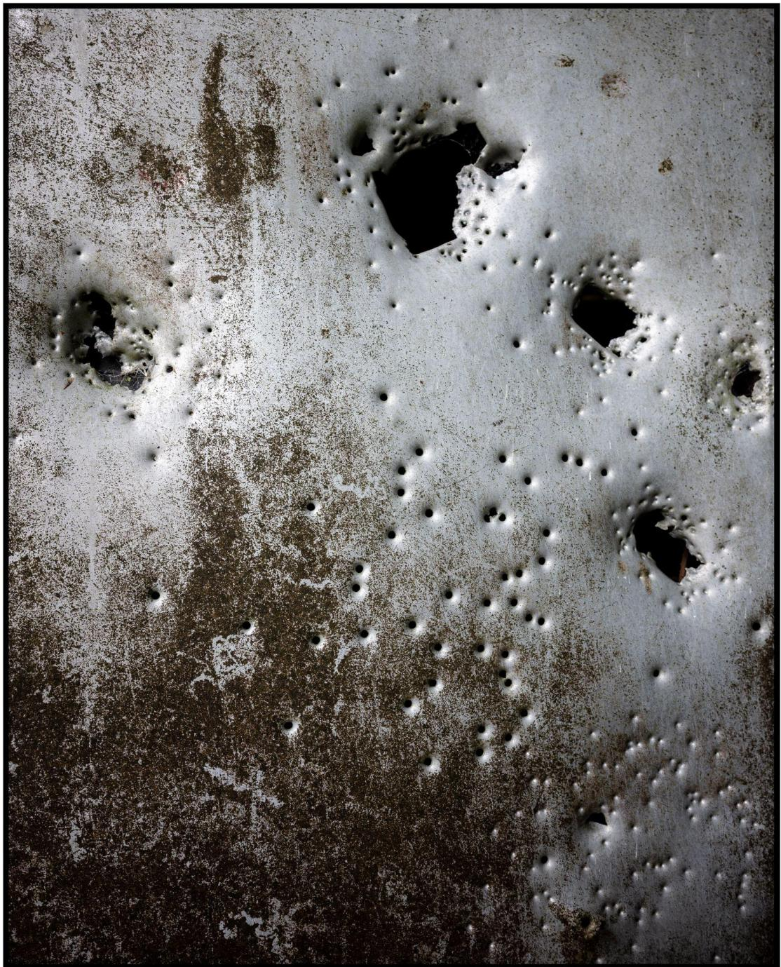
The large holes with small groupings were likely created by a close-range single birdshot while the more spread out holes are .22 groupings. The damage they can cause seemed very apparent on the side of this poor trailer.
